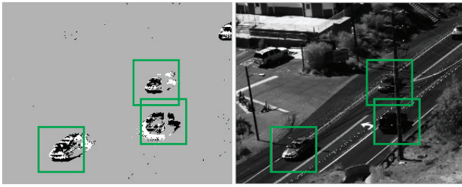
Fig. 2. Screenshot from live operation while tracking and identifying moving targets. Boxes indicate tracked objects, while colour indicates the object class (green indicates a car). The ATIS performs both change detection (left) and absolute grayscale measurements (right), but only change detection is used for classification, the grayscale image is shown just for visualization. Static objects are not detected (car in the top left), and objects overlapping the scene border are ignored (top right). All three objects moving within the scene are accurately tracked and identified, even though two are partially obscured by a lamppost.
